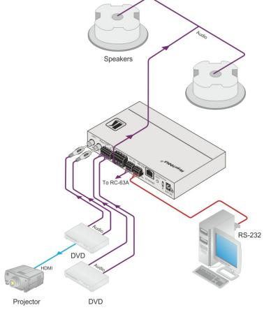
Figure 1: SPK-C612 in a Boardroom Setup
